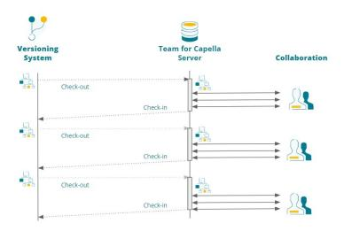
Users can simultaneously edit the same Capella model without conflicts. Only modified elements are locked, not the whole model, and other users can see in live modifications made by connected
